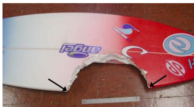
Fig. 5 Bite damage to a surfboard produced by a large tiger shark ( Galeocerdo cuvier ) during a traumatic injury attack upon a human in Hawaii. The bite circumference (ends shown by arrows) was measured on the photograph to be 645 mm. The size of the shark responsible for the damage was predicted, using the upper jaw circumference equation in Table 3, to be 4,486 mm in total length. See text for additional details (Case Study). Photograph: R. Honebrink
