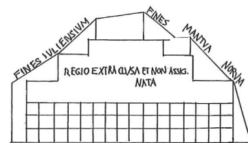
Centuriation and "excluded" lands and boundaries, with two neighboring coloniae (Mantua and Colonia Julia). Illustration of a surveying exercise by Hyginus Gromaticus, corpus agrimensorum [after O.A.W. Dilke, The Roman Land Surveyors (London, 1971), Gli agrimensori di Roma antica (Bologna, 1988), fig. 15.]
